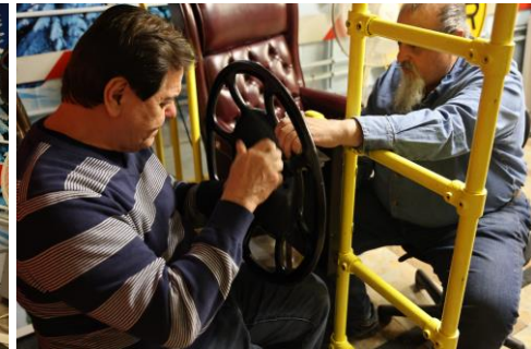
Joe, Tom and Jeff rework the caboose brake wheel making it more robust.
